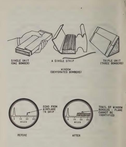
The drawings at the top of this page show typical bundles of "Window" while the "before and after" illustrations below indicate the way that the image on the enemy radar scope is confused by the strips of "Window" as they drop freely through the air.
